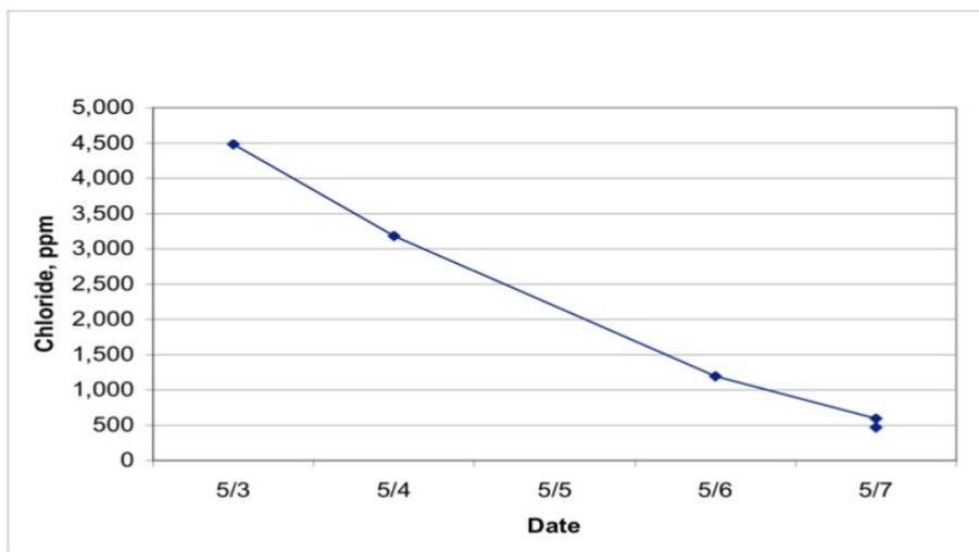
**Fig. 8 – Chloride Removal from a Gas Plant Amine**
