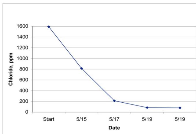
**Fig. 9 – Chloride Removal from a Refinery Amine**
