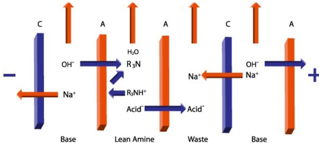
**Fig. 2 – The ElectroSep Electro dialysis Process**
