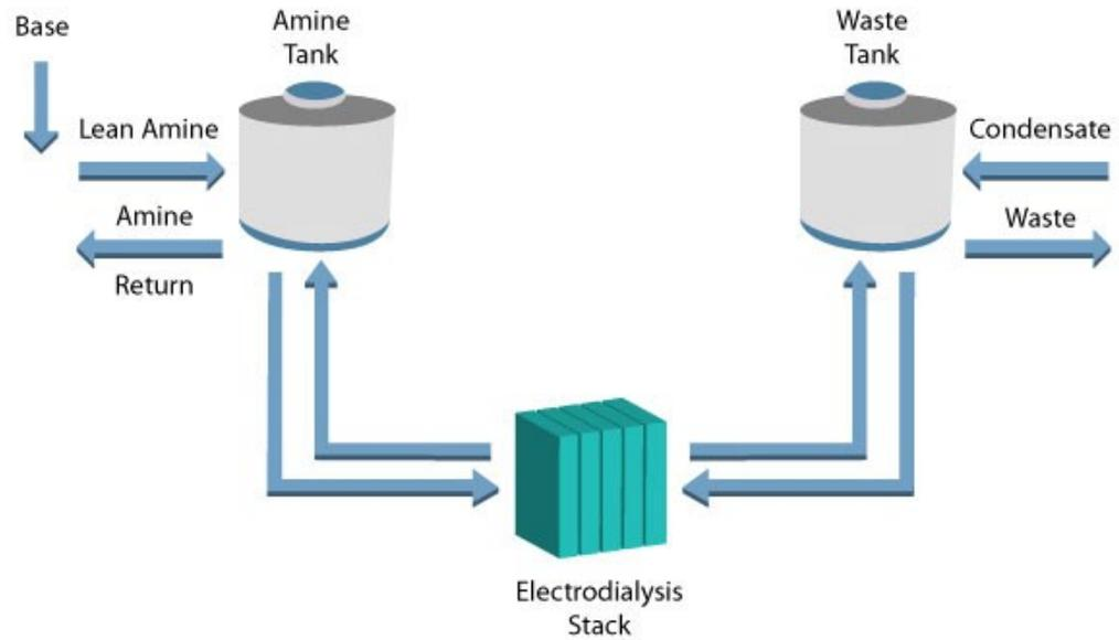
**Fig. 3 - UCARSEP Process Flow Arrangement**
