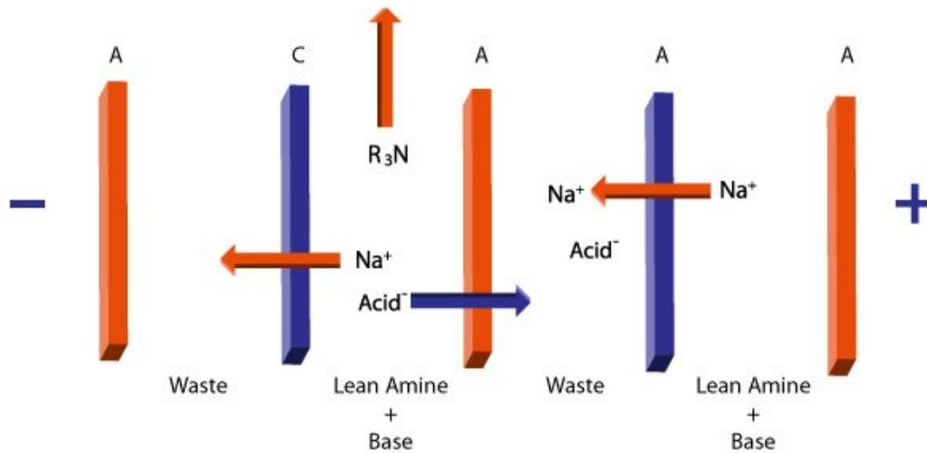
**Fig. 1 - Principles of UCARSEP Electrodeialysis Process**
