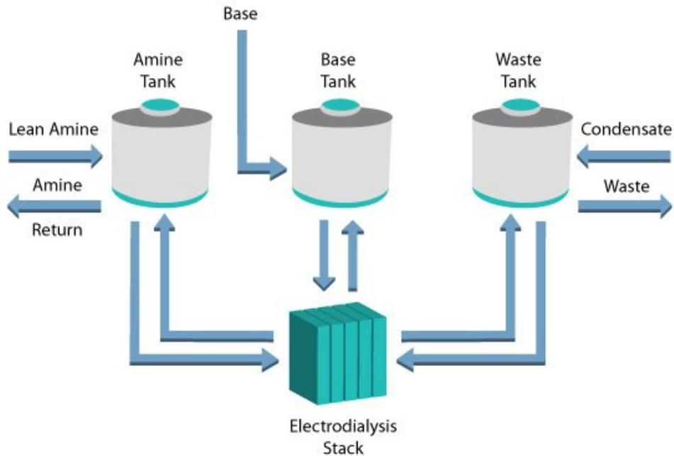
**Fig. 5- ElectroSep Process Flow Arrangement**
